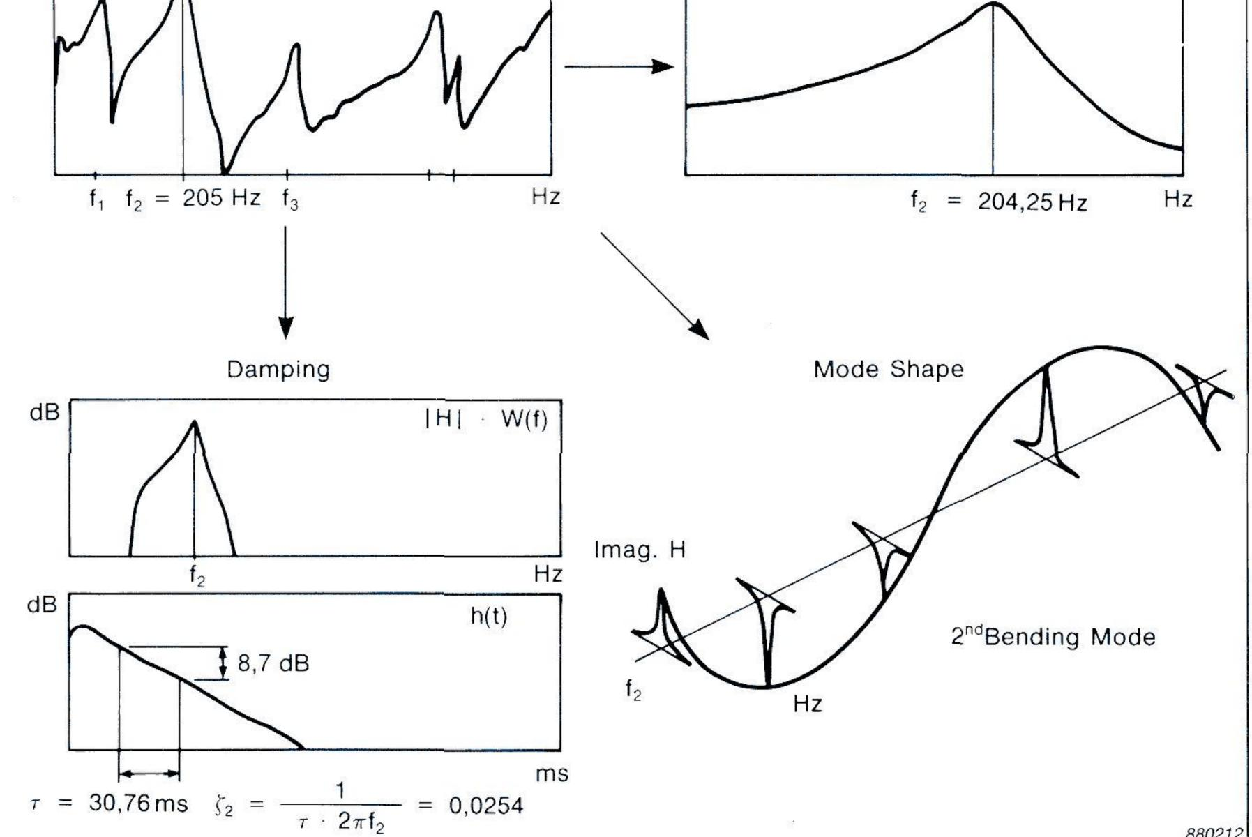
The frequency response function of a structure can be separated into a set of individual modes. By using a Dual-Channel Signal Analyzer Type 2032 or 2034, each mode can be identified in terms of frequency, damping and mode shape.
