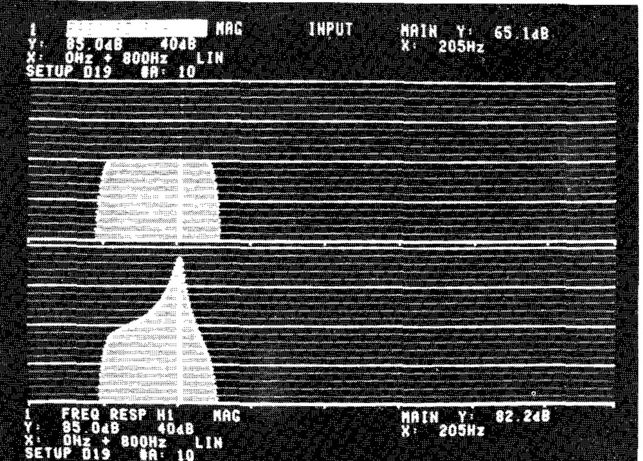
Fig. 5. Determination of the damping for the second mode by indentification of the half-power points.
