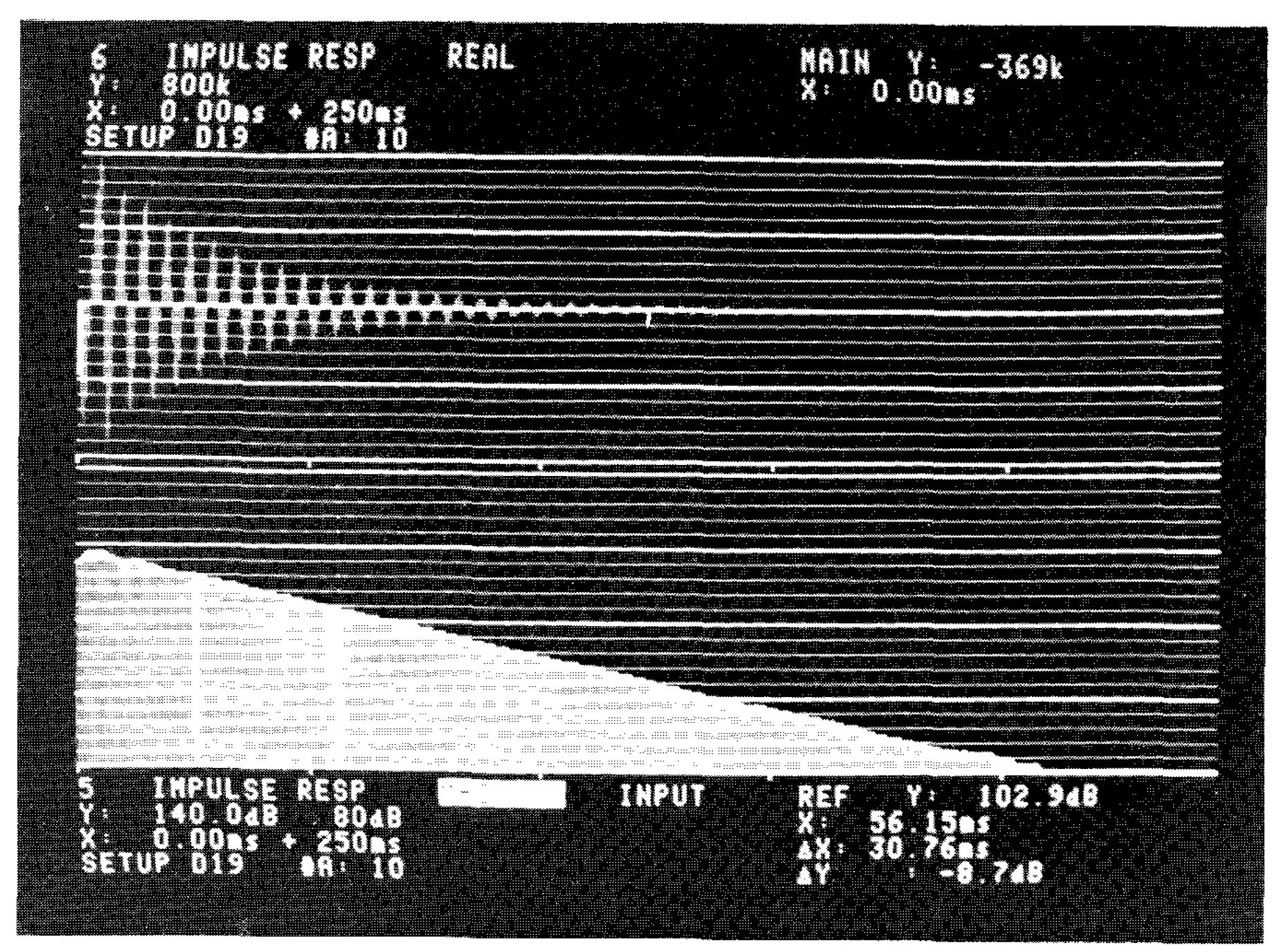
where  $\Delta f$  is the frequency bandwidth between the two half power points. The use of the analyzer's reference cursor greatly simplifies the determination of the bandwidth  $\Delta f$ .
